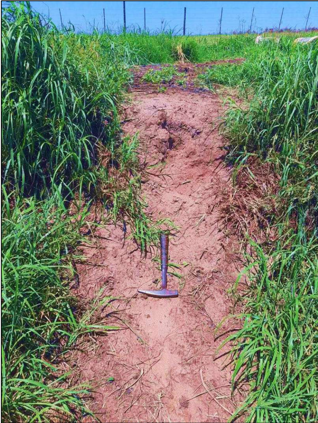
Figure 11 Geo-pick indicating the thickness of the topsoil layer.
